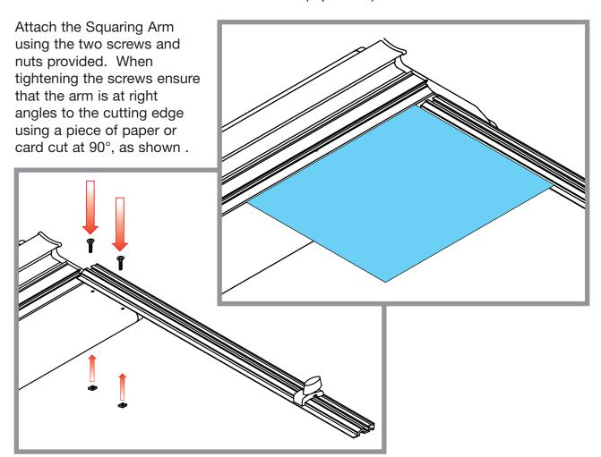
To fix the scales in the correct position, place a piece of card on the Squaring Arm and slide the measuring stop to the back corner then fasten it in position. Cut the card by depressing the blade and drawing it through the card smoothly. Measure the width of the card, and stick down the measuring scale so it reads the measured dimension at the stop.
