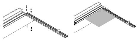
To fix the scales in the correct position, place a piece of card on the Squaring Arm and slide the measuring stop to the back corner then fasten it in position. Cut the card by depressing the blade and drawing it through the card smoothly. Measure the width of the card, and stick down the measuring scale so it reads the measured dimension at the stop.
