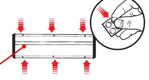
Rubber feet to be equally spaced along left and right edges of the base.
