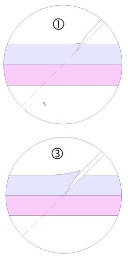
Replacing the double edged blade with a single edged or chisel edged blade will follow a straight path as the right hand side of the board does not have to move or shrink back by half the thickness of the blade.
