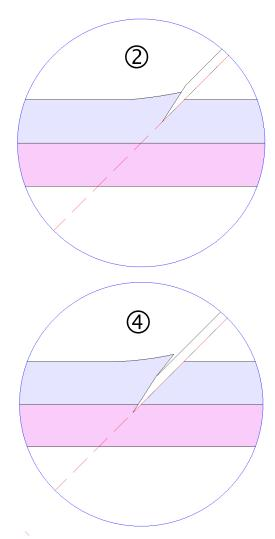
Care needs to be taken when using single edged blades that they are loaded into the cutter in the correct way, if the wrong tip of the blade is used the flat face of the blade will be uppermost so the right hand half of the board will push it away even more than it does with a double edged blade.
