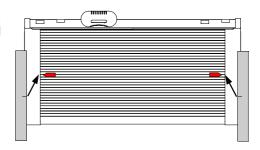
Remove the red protective cover from the fixed blade before use.
