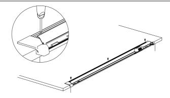
Fix a piece of 3mm MDF, PVC foamboard, or similar material to the table top as shown to bring the table surface in line with the base plate level of the Cutter.
