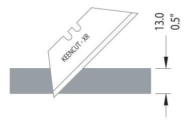
Consideration should be given to the toughness of the board being cut and the maximum depth of cut. For ease of operation it is recommended that dense materials such as PVC foamboard should not exceed 6mm (0.25") in thickness. Lighter materials, such as foam centred board can be cut up to 13mm (0.5") thick using the KEENCUT XR blade.
