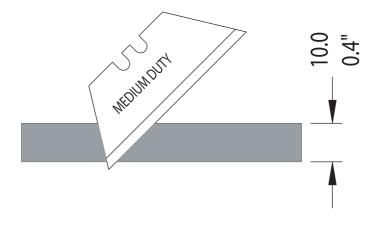
An increased cutting depth of 13mm (0.5") requires the KEENCUT XR utility blade available from Keencut distributors.
