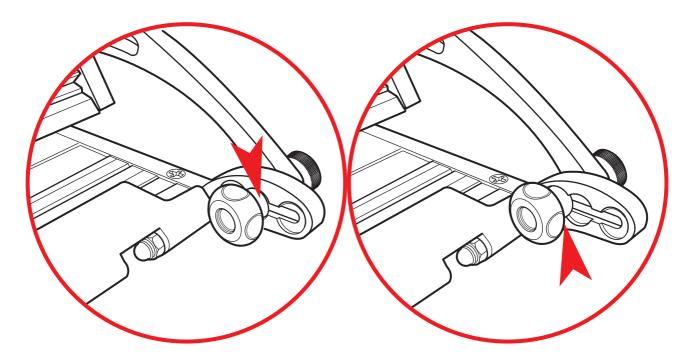
The third (furthest) position is also for cutting textile but uses a different part of the Cutting Strip should it become worn. The Cutting Strip can also be removed, turned around or flipped over to allow eight tracks to be used before the strip requires replacement. Replacement Cutting Strips are available from your Keencut agent.
