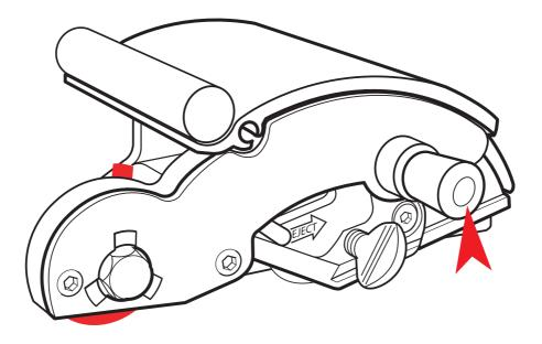
Position the textile on the machine and lower the Cutter Bar. Rotate the red safety guard into the cutting position, lower the Cutting Head until the circular blade makes contact with the textile and will cut cleanly without any excess pressure. Using steady pressure cut the textile in one smooth motion.
