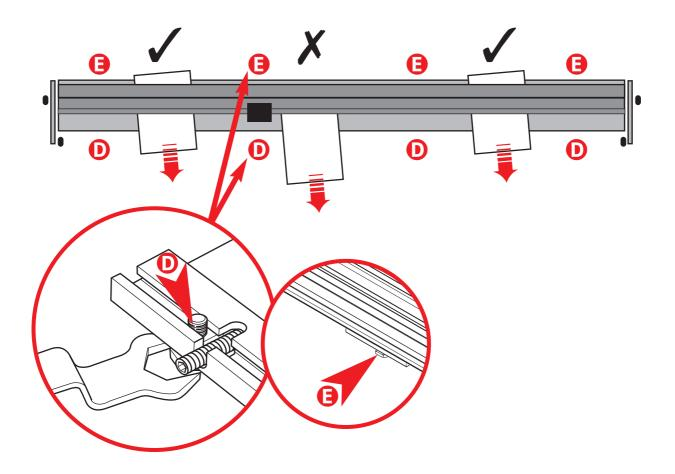
Adjust the clamping by turning the Jacking Screws "<sup>[]</sup> & "<sup>[]</sup> in the Base Fixing Brackets that are adjacent to the areas that are not clamping the paper. Turn the Jacking Screws clockwise (as you look down on them) using the wrench supplied, turn both the front and rear Jacking Screw by the same amount (to keep the Bracket level) until the paper is gripped. You may find that two or three adjacent Brackets need adjusting if you have a wide area that does not clamp.
