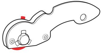
First raise the Cutter Bar using either Lift & Hold Lever, then loosen both of the Hinge location screws until the underside of the screw clears its location recess. Push the Cutter Bar until the underside of the location screw is positioned over the middle recess and tighten Hinge location screws. Repeat at the other end. The Cutter Bar is now positioned over the plastic Cutting Strip.
