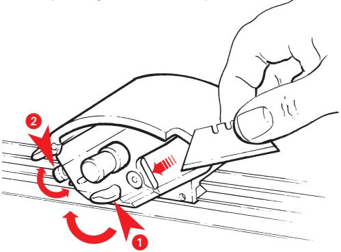
**TIP** - Set the blade depth with the tip protruding through the material just enough to cut consistently along the full length. A blade set too deep requires much more effort when cutting dense materials.
