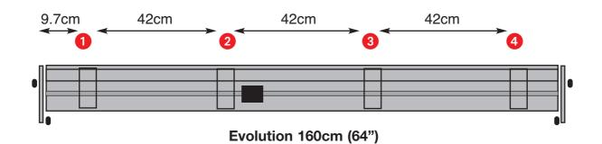
Lift the Evolution cutter bar from its crate **but** <u>do not remove the clear plastic stretch-</u> <u>wrap bands</u> holding the base to the cutter bar. Place the Evolution centrally on the Brackets and manoeuvre it until the base is located properly down on each of the Brackets.
