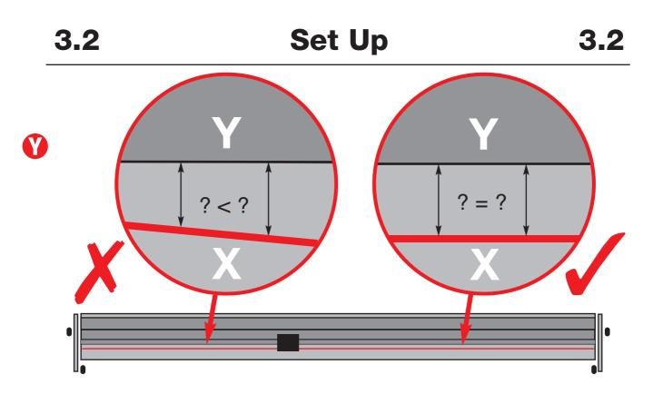
Adjust the straightness of the Base by adjusting the front "()" and rear "()" grub screws in the Base Fixing Brackets:
