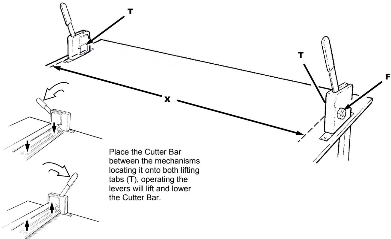
Loosen the friction knobs (F) on each of the mechanisms to allow the cutter to be raised, they can be adjusted to just hold the weight of the Cutter Bar. This enables the Cutter Bar to be held just above the surface of the material being cut for easy and accurate alignment.
