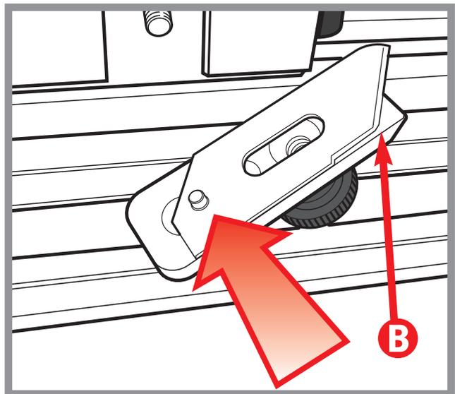
Hold the clamping plate in place on the blade holder and tighten the clamping screw ensuring that the blade is properly located in its groove.
