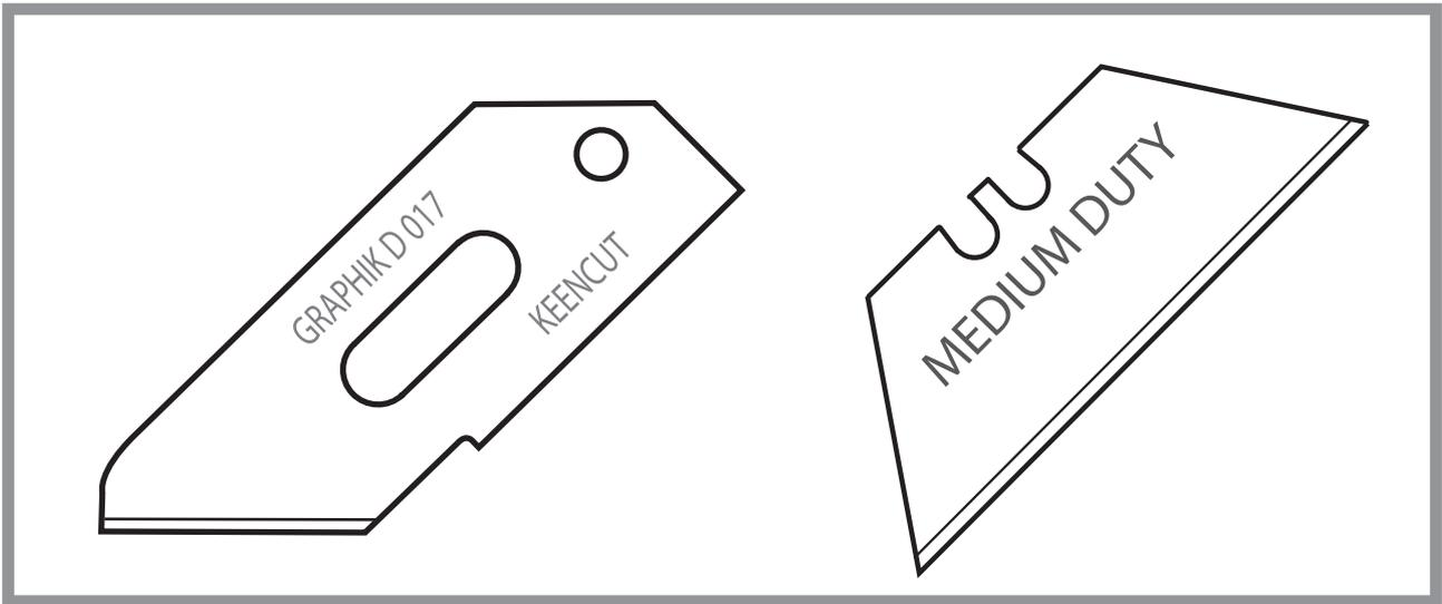
Consideration should be given to the toughness of the board being cut and the maximum depth of cut. It is recommended that heavy materials such as PVC foamboard should ideally be cut using the Graphik blade holder and to a maximum of 6mm (0.25") whereas, lighter materials like foam centred board can be cut up to the maximum cutting depth of the blade being used.
