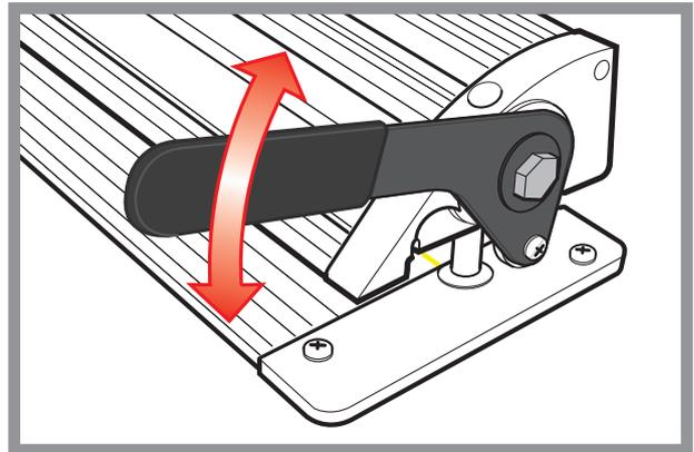
Lifting vertically remove the cutter from both guide rods at the same time. Check that the Base Plate is laying flat on the table surface along its length. If necessary use paper or card under the full width of the Integra base to make it level on a bench top that is not flat.
