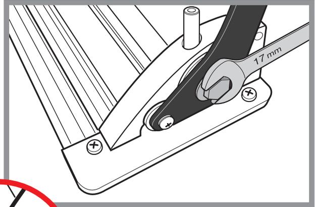
Check the cutter is in the correct position on the table and that the Base Plate and End Plates are in line.
