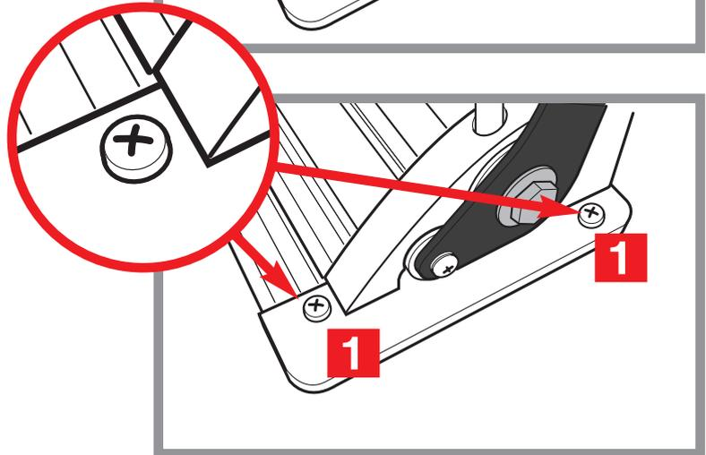
Attach the two End Plates using the four pan head screws **1**.
