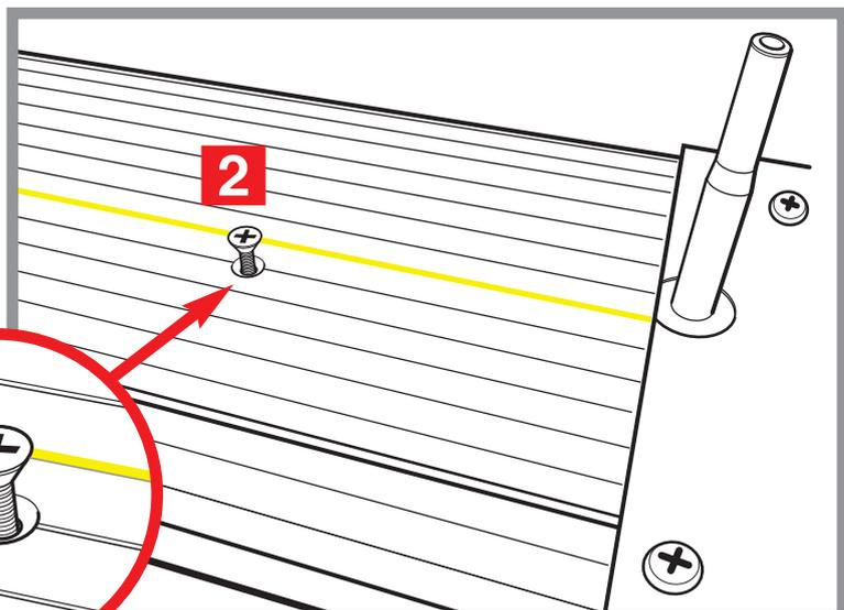
Use the countersink head screws **2** to fix the Base Plate to the table.
